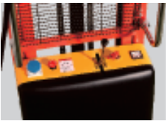
Precise lifting and lowering via hand lever. Battery cut –off switch prevents unauthorized use.
